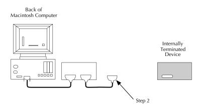
3. Position the Scanner so that you can connect it in the chain before the terminated device.
